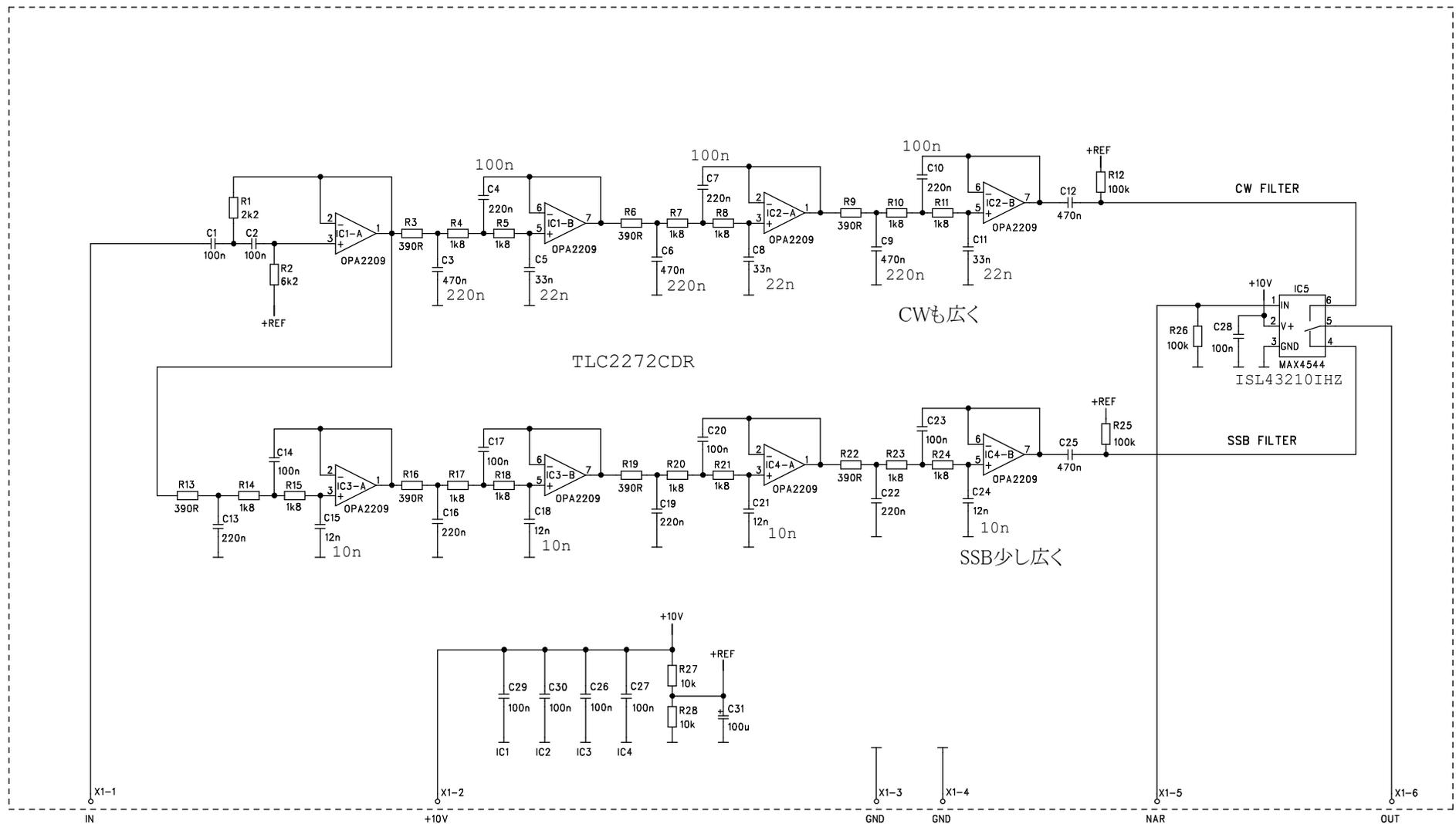
NOTE1: ALL OPAMPS PIN4 GND, PIN8 +10V.
